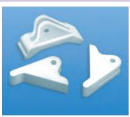
Designed for .062 (1.57) thick PC cards. Level action ejectors aids card insertion and extraction. Supplied complete with stainless steel spring pin.
